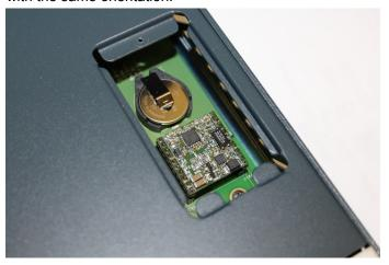
5. If there is a modem replacement, carefully lift the old modem out of its socket.
